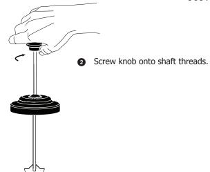
Place stir paddle into unit. Lift knob up and down to free clumped product.
